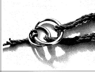
Smaller ring pulls up hard against larger ring when towing tension is applied.
