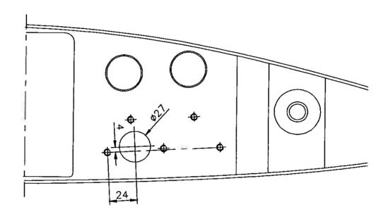
inspection opening in the outer wing rib (only for aircrafts with winglets)
