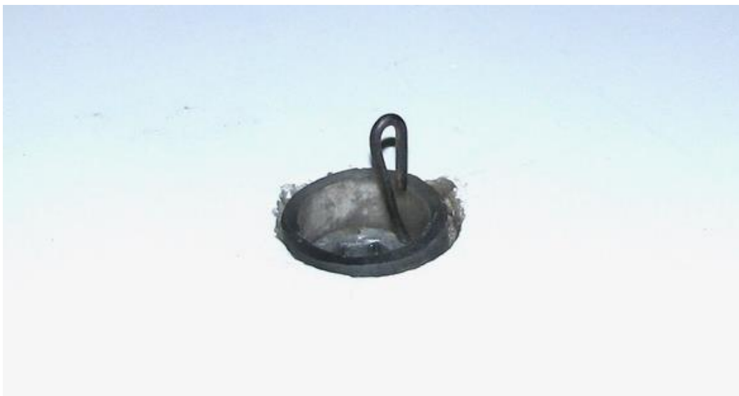
Figure 2: Vinyl Tube Inserted Over Safety Pin And Tailplane Retaining Bolt
