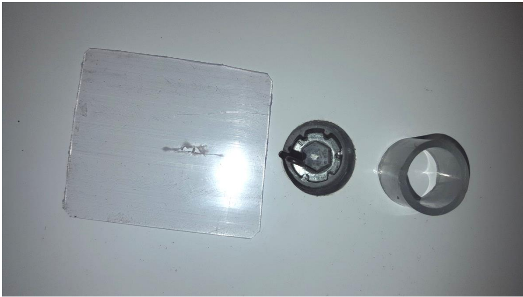
Figure 1: Vinyl Tube And Plastic Cover Adjacent To Tailplane Retaining Bolt
