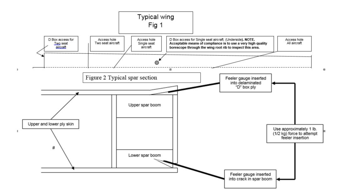
Through the inspection holes, inspect the internal structure of the wing trailing edge using a torch and mirror or suitable inspection equipment. Pay particular attention to the air brake box and drag spar attachment to the main spar.
