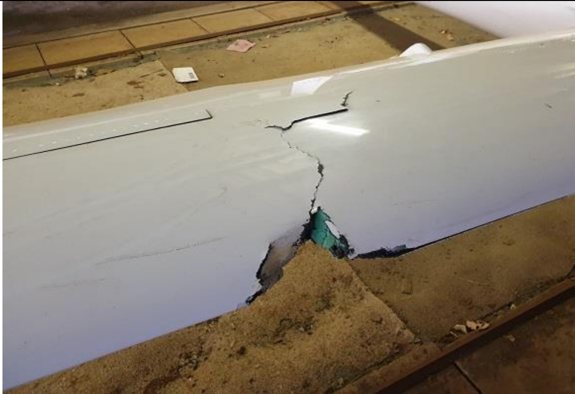
Fig 5. Starboard wing damage from impact with fence posts.
