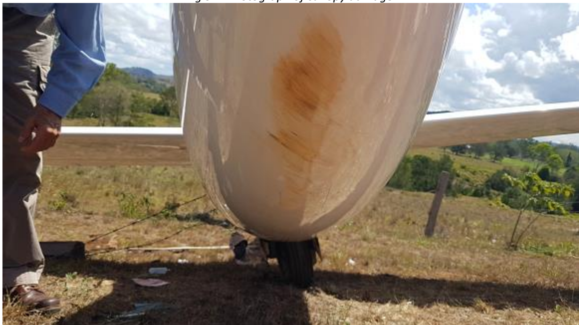
Fig 4. Fuselage damage from impact with rising ground prior to aerodrome boundary.
