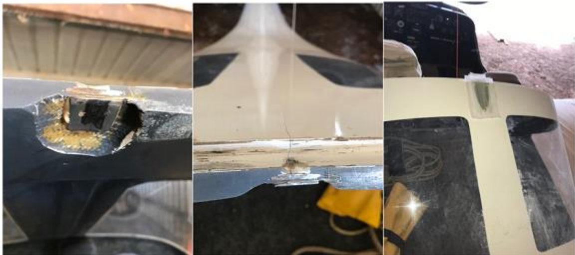
Fig 2. Damage to canopy locking mechanism
