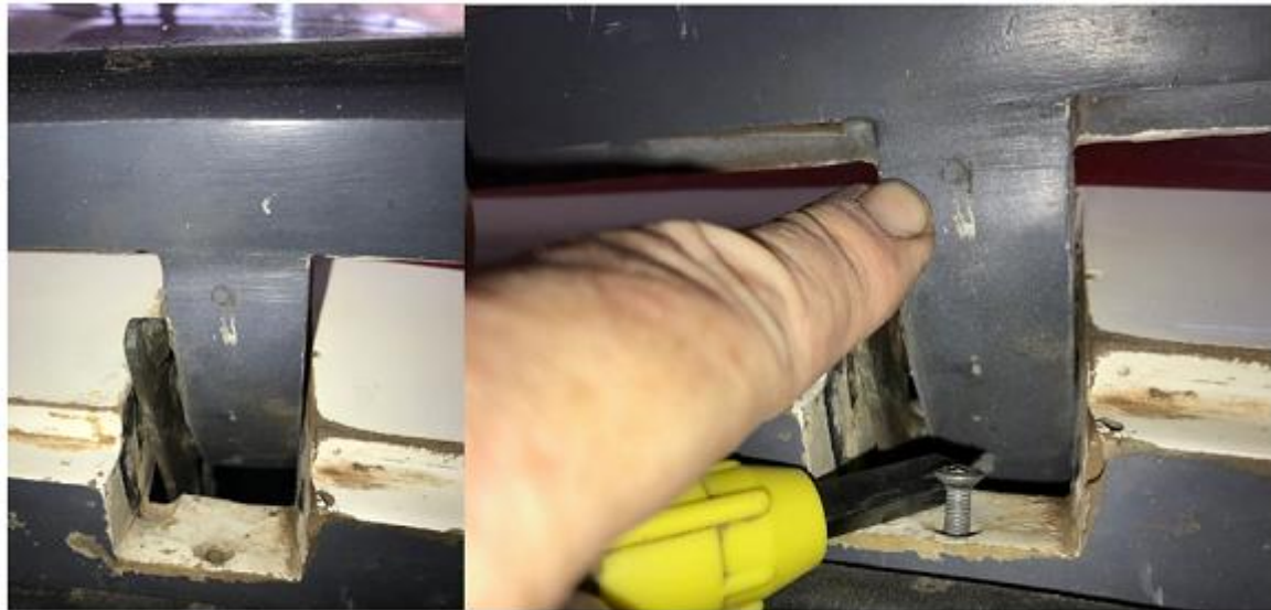
Fig 1. Canopy hinge showing wear from ill-fitting screws
