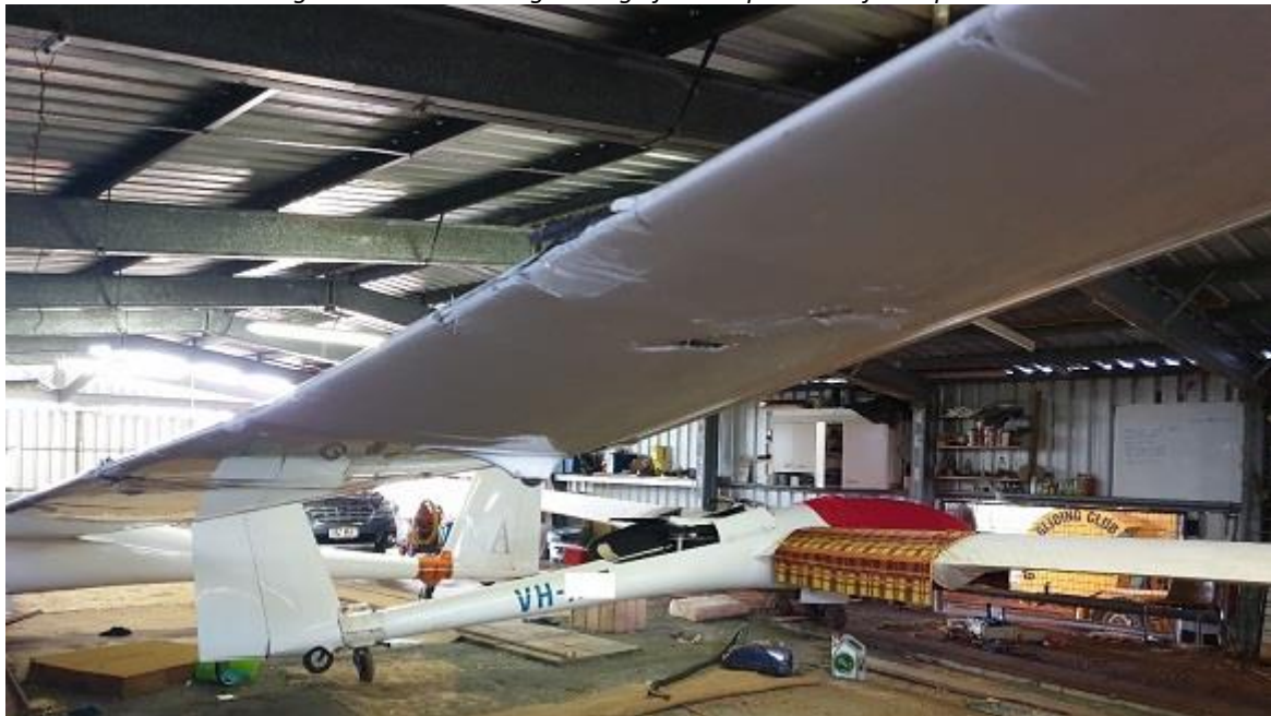
Fig 6. Port wing damage from impact with fence posts.
