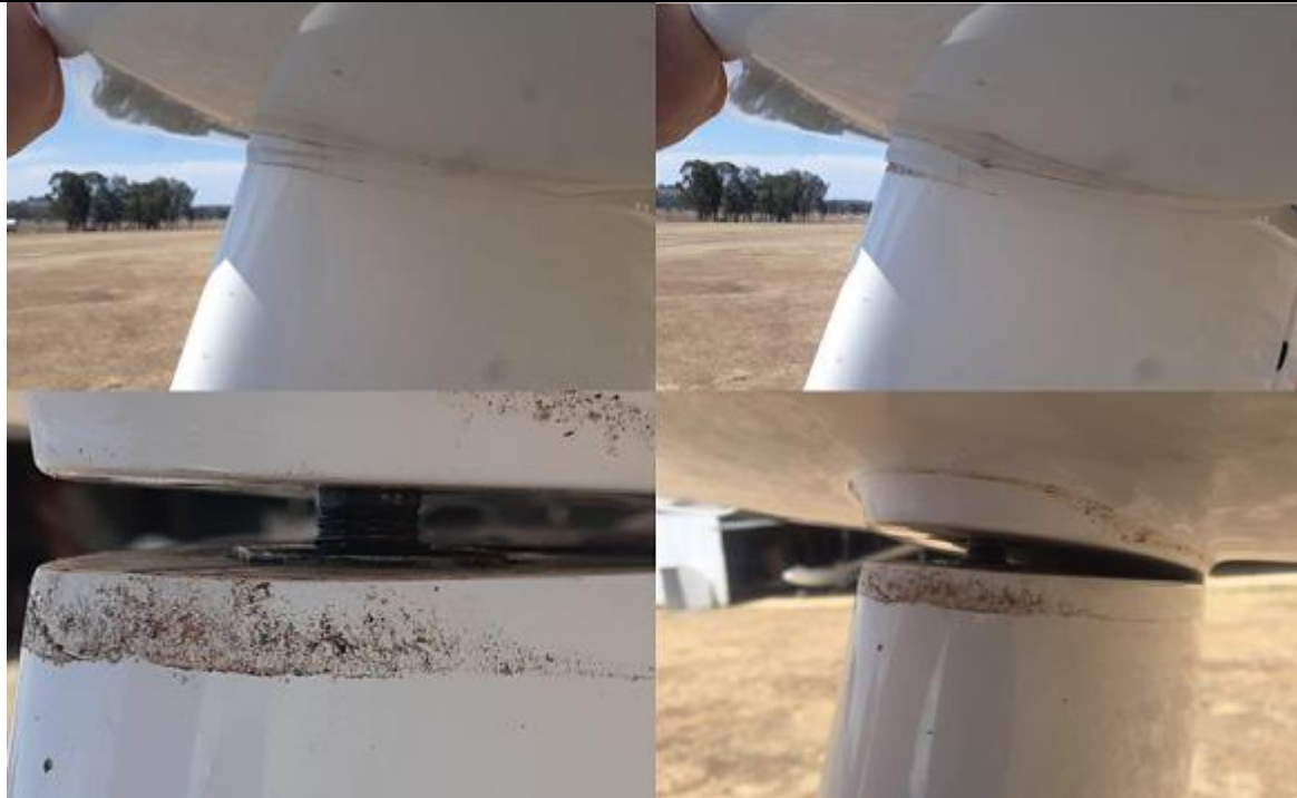
Pic 1 – Ill-fitted tailplane.
