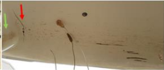
Photo 2 - Split behind the nosewheel fairing (red arrow) and scuff marks where the fairing hit the ground (green arrow).
