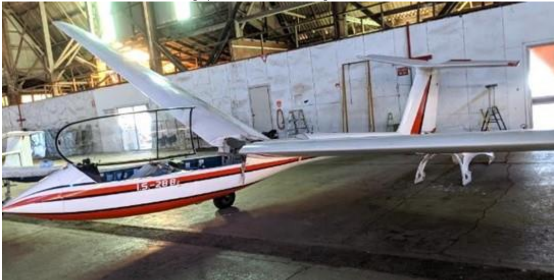
Photo 1 – VH-CQD Post Incident Showing Exaggerated Dihedral
