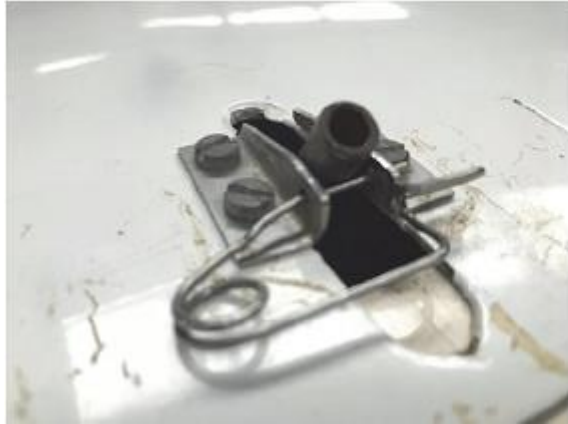
Figure 3. Position of locking lever and locking hooks with lever forward of safety pin. Note: only right hook shown.
