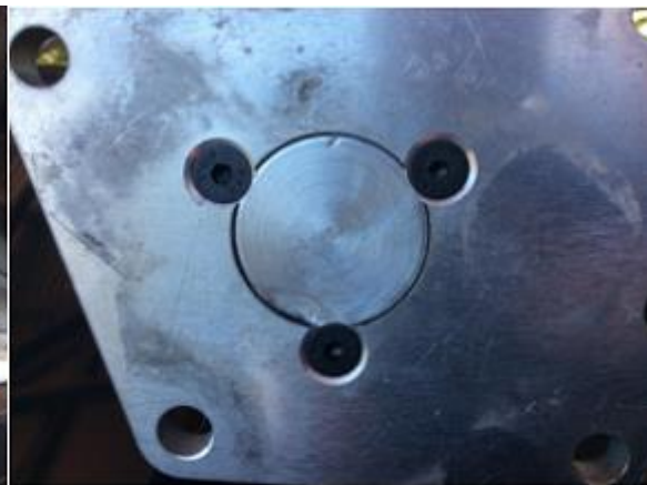
Picture 2 Dummy shaft mounting with new high tensile screws fitted.
