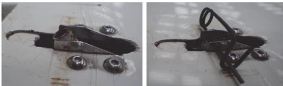
Figure 2. Locking lever when tailplane attached (left image) and when locked with safety pin inserted (right image)
