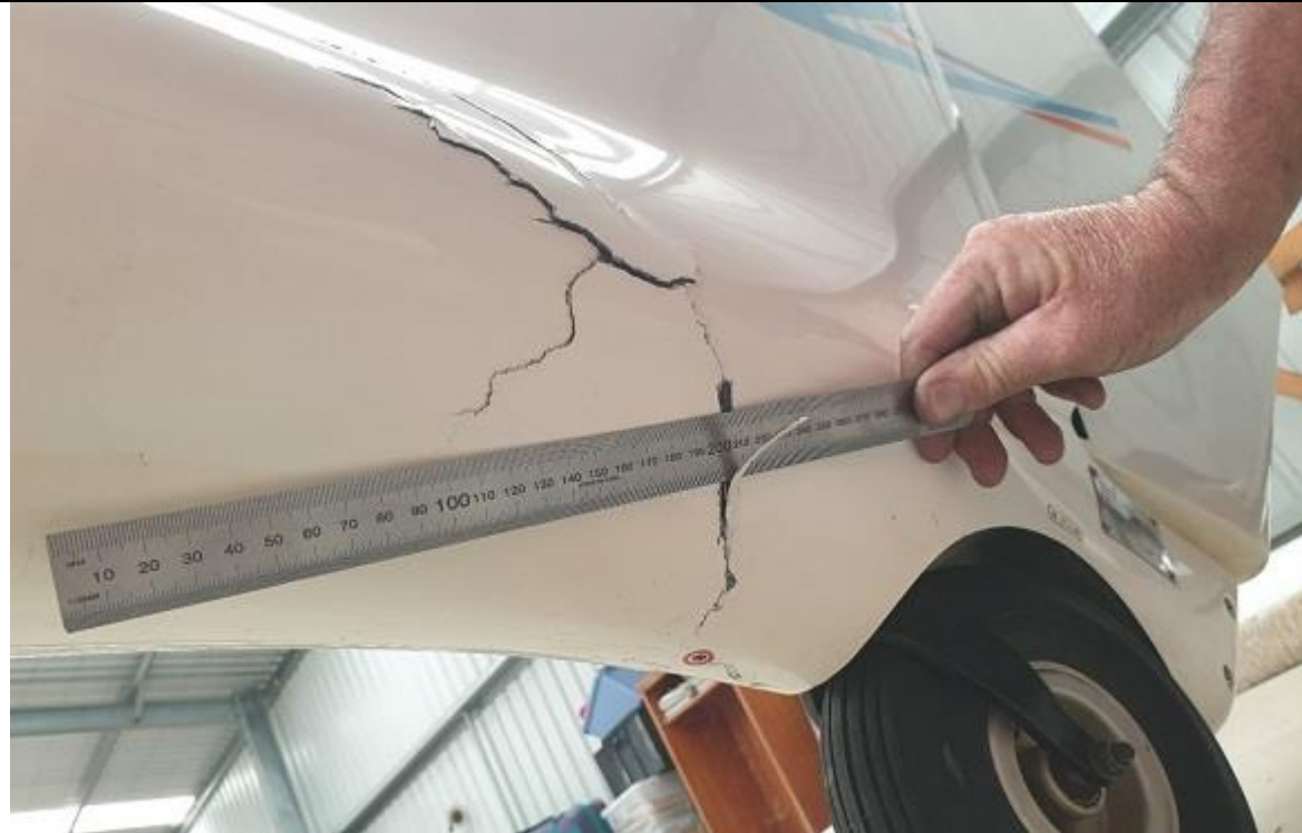
Figure 7: Full thickness fracture on the underside of the tail boom through to the port side.
