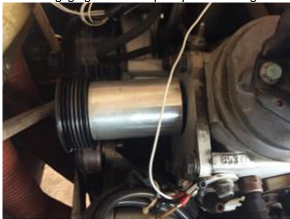
Picture 1 misaligned dummy shaft
