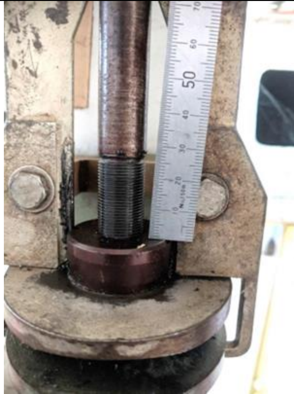
Photo 4 - Correctly engaged lower tapered bolt - 25 mm thread exposed, no wear / contact surfaces of tapered bolt exposed above upper surface of fitting, centre collar housed in retainer.
