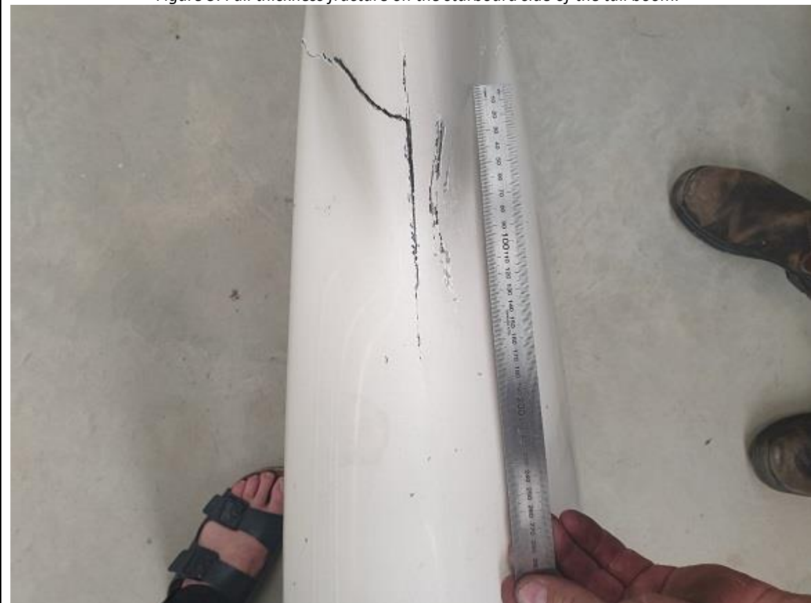
Figure 6: Full thickness fracture on the lower vertical stabiliser.
