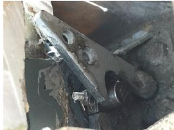
Figure 3. Position of locking lever and locking hooks with lever forward of safety pin. Note: only right hook shown.
