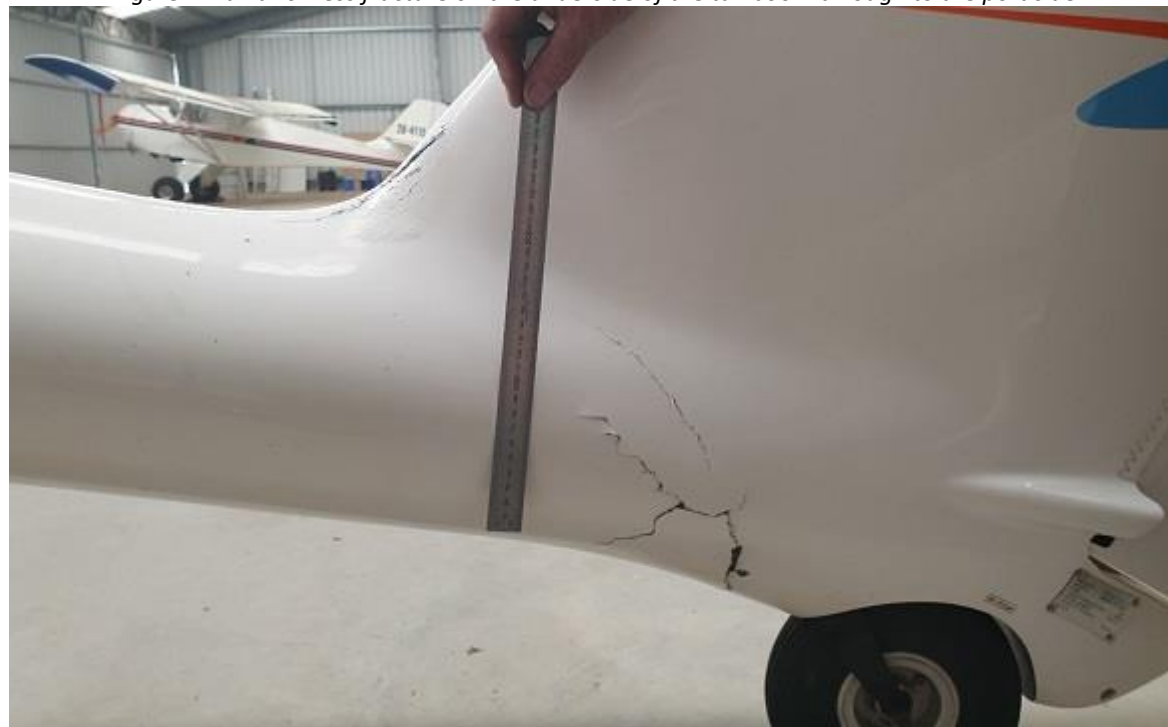
Figure 8: Full thickness fracture on the port side of the tail boom.
