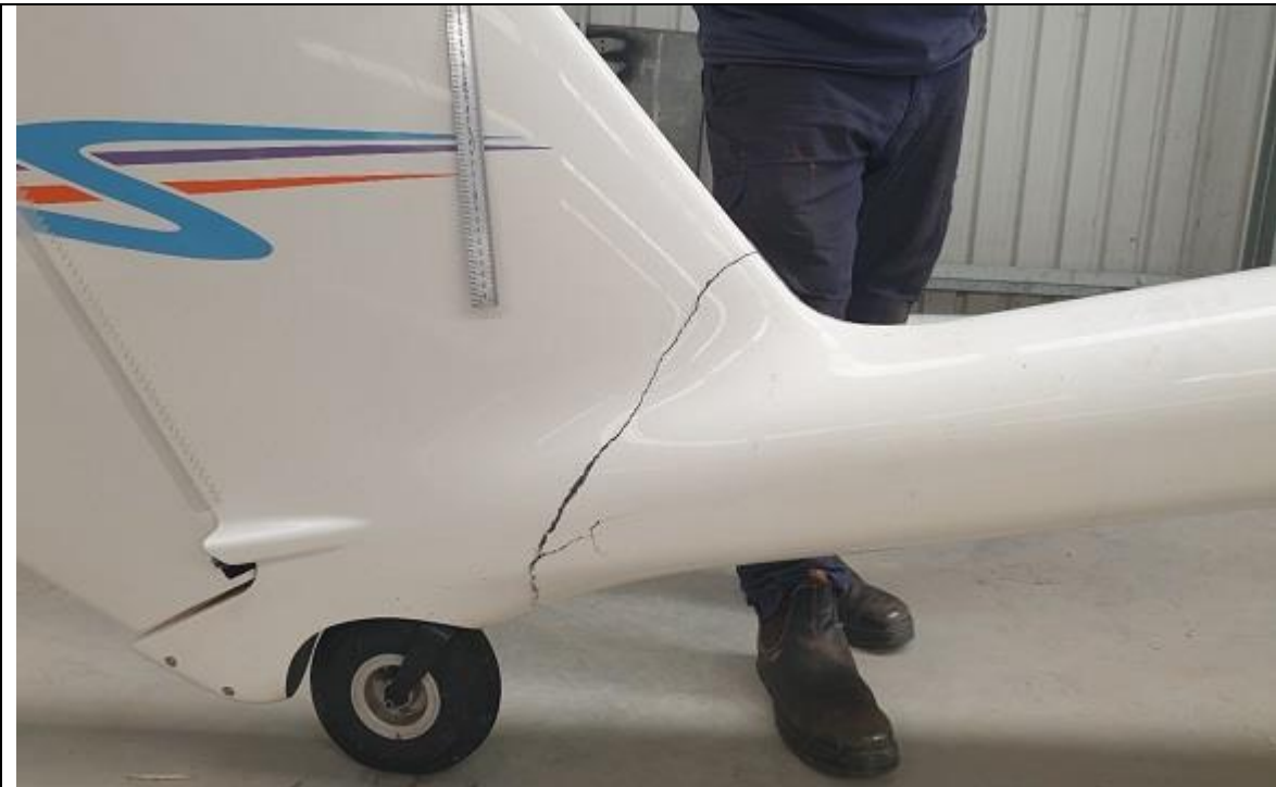
Figure 5: Full thickness fracture on the starboard side of the tail boom.
