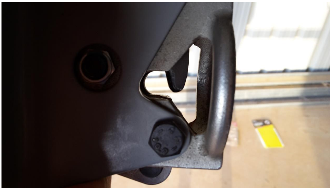
Figure 1: TOST E 22 release. Beak when fully closed has 3mm gap
