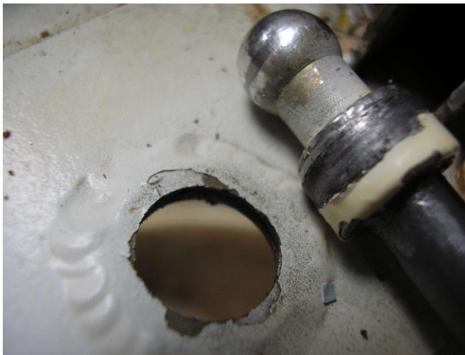
Photo 2. Left hinge pin failure area.
