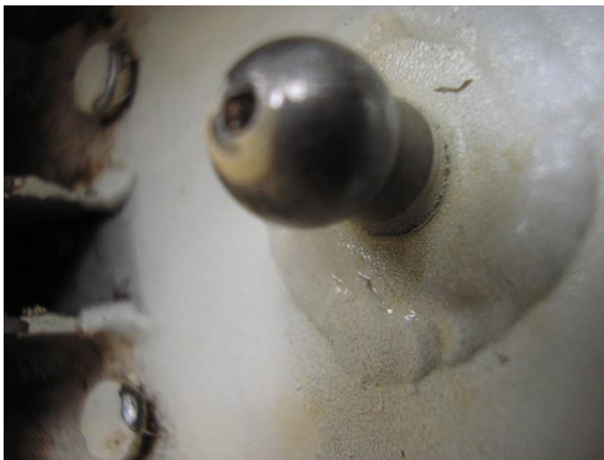
Photo 3. Right elevator hinge pin showing cracking around 40% of the circumference.
