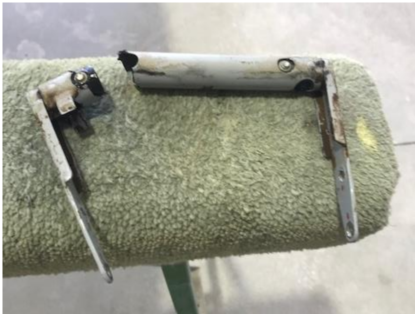
Figure 1: The affected sailplane on the daily inspection showed excessive lateral play. With the failed component installed, the crack looked like only the surface finish was cracked. The crack is therefore very insidious and requires a thorough inspection. Any surface finish defects around the holes in the torque tube should be treated with suspicion and investigated further.
