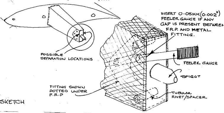
2. If any separation between the fibreglass wrapping and the stub end metal fitting is detected insert a 0.05 mm or 0.002 inch feeler gauge into the gap between the fibreglass and the metal fitting to check the depth of separation but do not force the feeler gauge into the gap.
