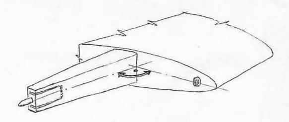
1.4. Preserve the "old" pin situation in respect to the spar root geometry by means of 11-90-00/Px4 tool or the auxiliary tool of wood or plywood as shown on the sketch below.
