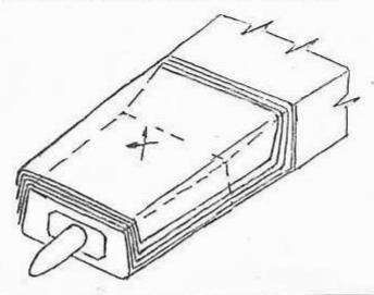
4.5. Check the condition of the whole set, prepare the surface and wrap on the distance of 115 mm from the spar root 120 bounds of ER 2003 roving and than glue in the covering item 23 and 27 of drawing No 11-90-00 and 11-91-00, providing that the 27 covering lenght ought to be 270 mm. Cure under the pressure applied at the "oblique" wall side to ensure the assembling play.
