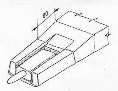
Clean and smoth the composition flows after the "block" is glued up - clean the chamfer between the longerons for the compensating fabrics.
