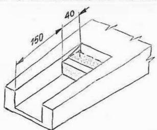
2.3. Prepare the "block" with pin for glueing: remove the grease using the extraction gasoline, grind the surface covered with BWF-21 glue using the sand paper of 220 grade with the cross-way motions (avoid to damage the glue layer) - remove the dust of the whole set.
