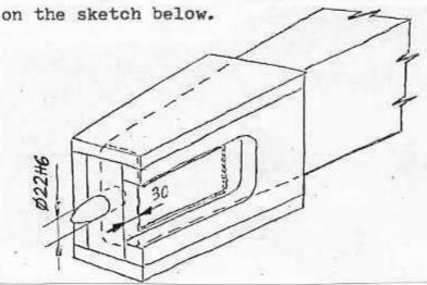
1.5. Sperate the pin out of the "oblique" spar wall by means of drilling with the long drill paralely to the pin axis (in case the auxiliary tool is used it should be removed out of the spar). Remove the "old" pin tearing it out of the wall.
