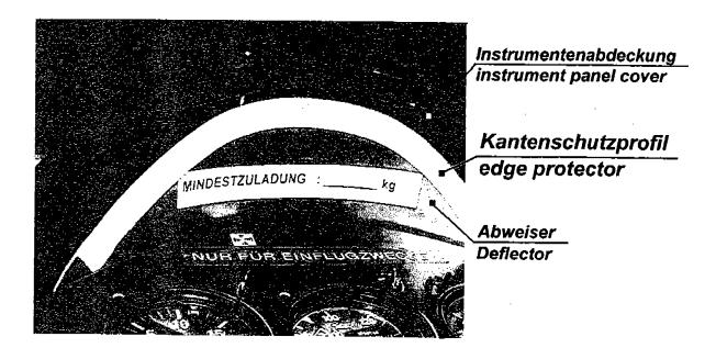
Should the instrument panel cover be too short to allow the protector to fit underneath, contact manufacturer stating model and serial number.
