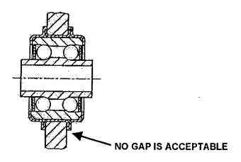
**DETAIL "B" - BEARING FITTING**
